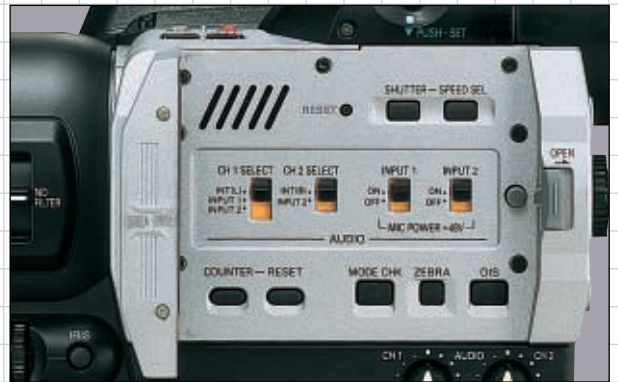
Sub-panel (with LCD monitor opened)
